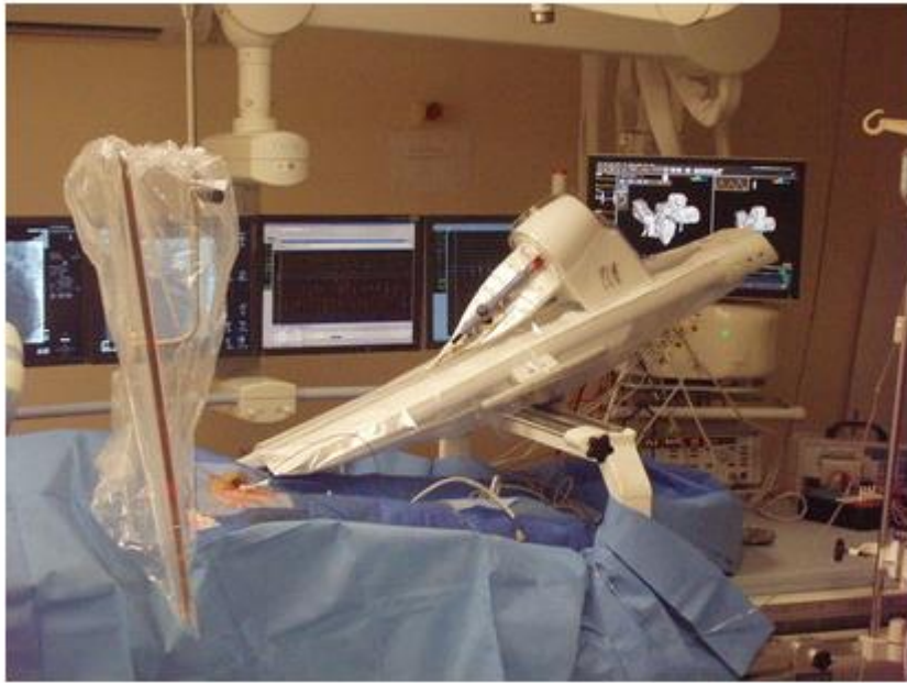
The Amigo robot with the navigation map and force displayed behind it
